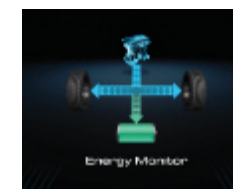
SERIES HYBRID: Driven by motor, charged by engine
